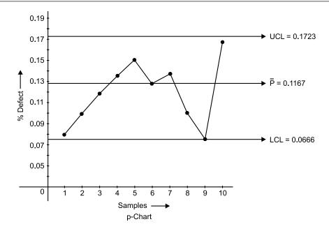
Upper Control Limit, UCL =  $\overline{p} + 3\sqrt{\frac{\overline{P}(1-\overline{P})}{n}}$
