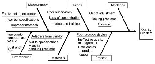
Fig. 6.3 Fishbone diagram
