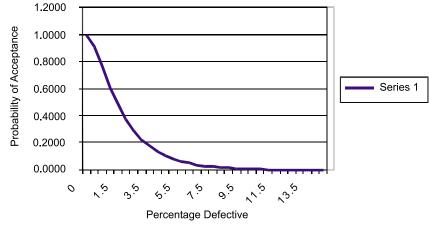
Fig. 6.9 Operating characteristic curve
