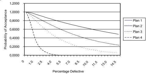
Fig. 6.10 Operation characteristic curve for different samples.
